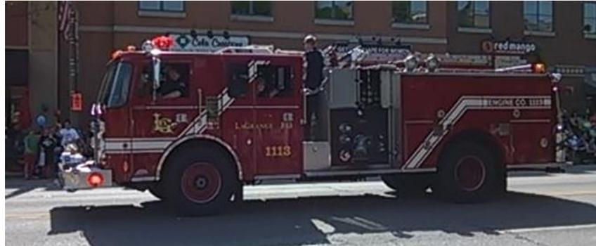
Engine Co. 1113 is a 1991 Pierce Lance fire engine. The vehicle is equipped with a 1500 gpm pump and 500 gallon water. This vehicle still serves the residents of La Grange today.
